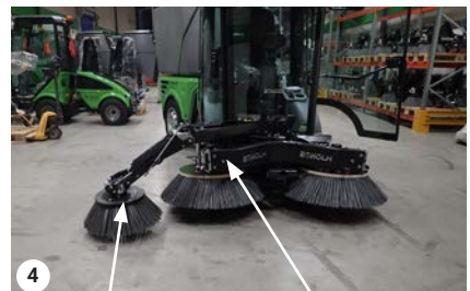
Kippen (linker Joystick) Arm bewegen (rechter Joystick)
