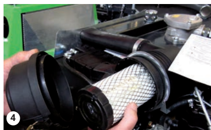
Luftfilterelement tages ud
