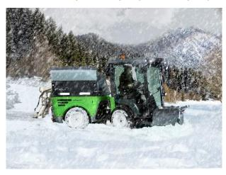
City Ranger 3070 is a large compact and multifunctional utility machine. With a total weight of 3 tonnes, an engine capacity of 67 HP and a new innovative sweeping system, the machine has become the preferred choice by many actors within the field of urban cleaning.
